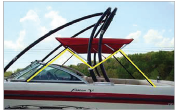
Placement of the hold-down straps should form the letter "M". Straps should form a 45 to 90 degree angle with each bow.
